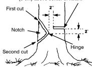
After removing the wood from the notch, make the felling cut on the opposite side of the notch. This is done by making a cut about two inches (5 cm) higher than the center of the notch. This will leave enough uncut wood between the felling cut and the notch to form a hinge. This hinge will help prevent the tree from falling in the wrong direction.
